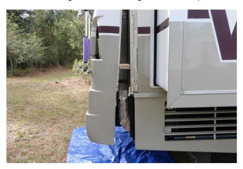
And then just grab the bottom edge of the cap and start pulling. Have a couple of blocks handy to prop it open. At one point I had the bottom edge of the cap out about 18". I kept checking the top of the cap to make sure it was not moving. Now you can remove the ducting.
