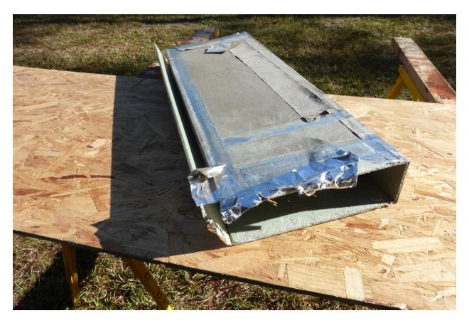
Isn't this lovely? All I had done to this point was remove the duct. The only thing holding it together was the tape at each end where it connected to the plastic plenums. The tape along the joint fell off while I was removing the duct.
