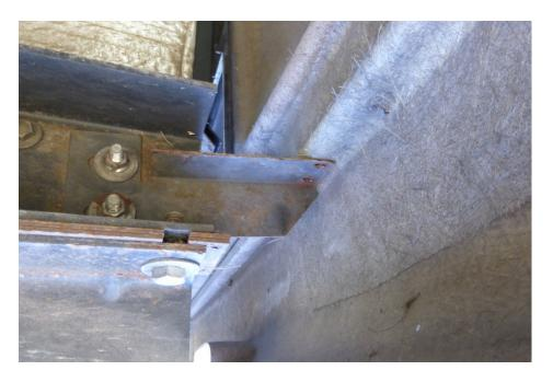
At the end of the frame rails. There are also two screws that hold on the third brake light to a stand-off bracket. The intake/exhaust port for the furnace will also need to be removed. There may be other connection points on your particular coach. You'll know if you missed any as soon as you try pulling out on the bottom of the cap. I also removed the tail lights to allow more light behind the cap, but this is optional.
