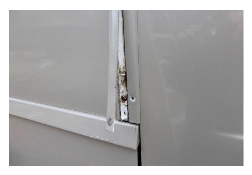
The trim pieces on each side will need to be removed. The center strip is held on by a double sided tape. I had to order tape from Amazon to reinstall the strip (TapeCase
